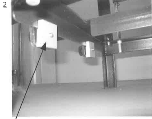
Install Rail Mounting Blocks and Thumbscrews as shown. Do not tighten.
